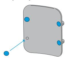
**3.** Apply a liberal amount of Fabtech +PLUSeries® 60 Second Adhesive or similar to the rear surface of the Socket Plate and press onto socket at determined mounting location. Hold in place until adhesive has cured.
